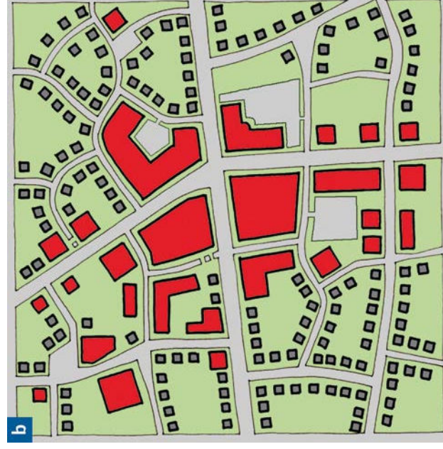
Figure 6.1: In typical post-WW2 developments (a), the main roads are often the only through routes. In more historic areas (b), there may be quiet parallel routes that could be made suitable for cycling (images from Manual for Streets)
