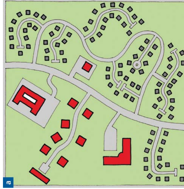
Figure 6.1: In typical post-WW2 developments (a), the main roads are often the only through routes. In more historic areas (b), there may be quiet parallel routes that could be made suitable for cycling (images from Manual for Streets)
